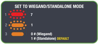
WIEGAND: FOR CONNECTION TO EXTERNAL ACCESS CONTROL SYSTEM PRESS \*\* TO EXIT PROGRAMMING
