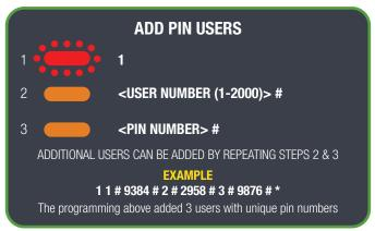
PIN NUMBERS MUST BE BETWEEN 4-6 DIGITS PRESS \* TO EXIT PROGRAMMING
