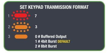
APPLICABLE WHEN IN WIEGAND MODE PRESS \*\* TO EXIT PROGRAMMING
