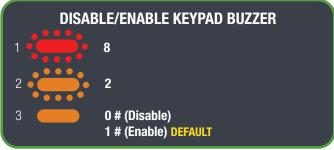
KEYPAD BUZZER WILL STILL OCCUR DURING PROGRAMMING MODE PRESS \*\* TO EXIT PROGRAMMING
