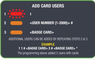
THE ABOVE METHOD IS PREFERRED FOR CARD PROGRAMMING SO INSTALLERS CAN NOTE WHICH USER NUMBER EACH CARD IS ASSIGNED TO.
